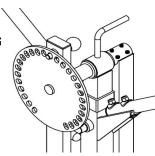
An additional pop-pin allows you adjust height for proper biomechanical function.
