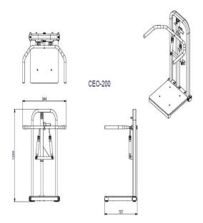
Side Bending Machine with hydraulic resistance mechanism
